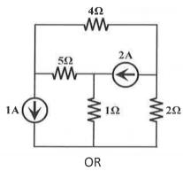
Q.2(B) Apply mesh current method, find the currents in resistances  $R_3$ ,  $R_4$ ,  $R_5$  and 10M 1 3  $R_6$  of the circuit shown in Figure.
